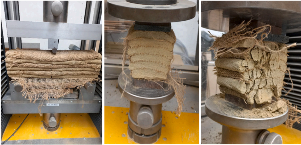
Fig. 4. Flexural and compressive strength test of 3D printed earth-based samples.
