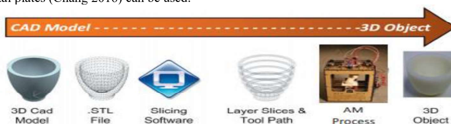
Figure 2. Generalized Additive Manufacturing Process (Campbell et al. 2011).
